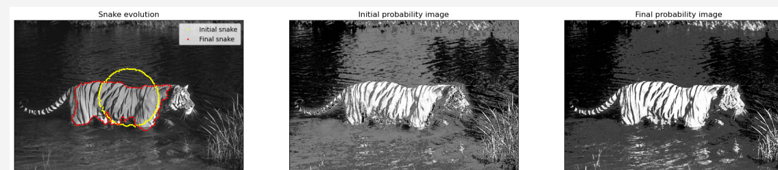
Figure 1: Initial and final snake (left), probability image with initial (center) and final snake (right). Implemented with 200 iterations and a stepsize of 3.
