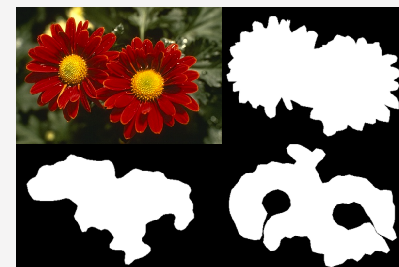
Figure 3: Flower (upper left), true mask (upper right), segmentation with standard parameters (patch size = 7x7, amount of iterations = 200, alpha = 0.01, beta = 0.1, and stepsize = 3) (lower left), and segmentation using more customized parameters (patch size = 5x5, amount of iterations = 250, alpha = 0.01, beta = 0.1, and stepsize = 10) (lower right)
